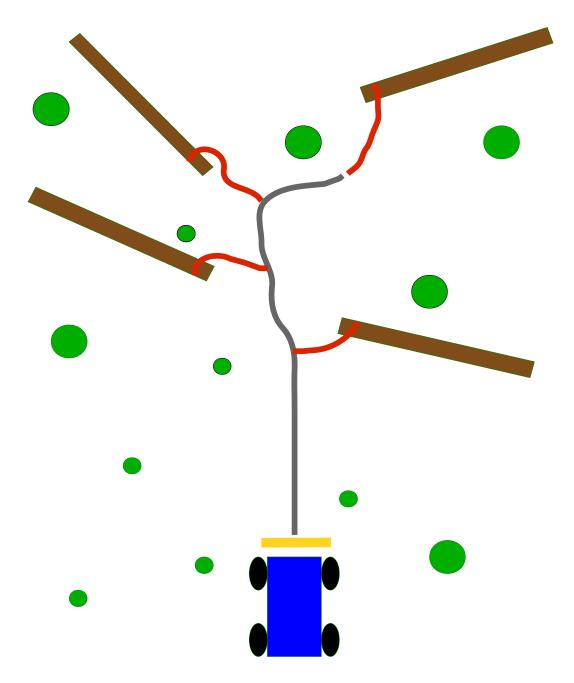
In this scenario, as the winch line (gray) is pulled in, the line will tend to straighten pulling the logs (brown) toward the center. As the end log comes in it will gather up the logs with chokers on sliders (red), which will straighten out and lay parallel to each other. This works best when the load on each side is balanced. Lighter logs that are not bound up in brush or coming uphill will move first.
