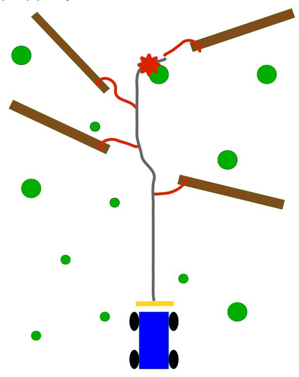
If a log gets hung up, it is usually best to stop pulling with the winch. It may just exacerbate the problem. The choker setter should communicate with the winch operator to stop and not try pulling again until the hang up is cleared. Hand signals or some form of communication is necessary to ensure that both workers are in safe spots before winching resumes.
