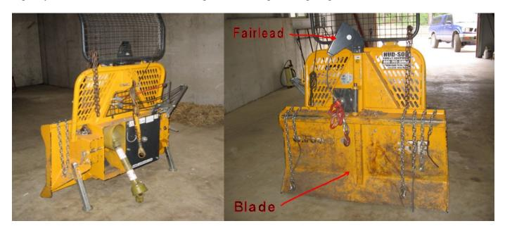
Skidding winches at the small end of the scale are usually driven by the tractor's PTO. Control ropes are used to engage the clutch and brake. The width of the 'blade' should be wide enough to extend from
