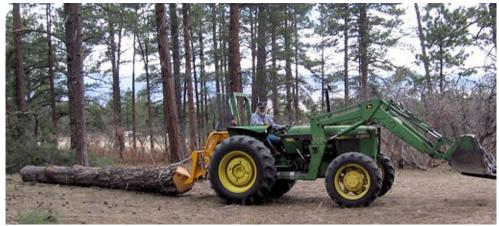
Representative of the mid-sized equipment is this 60 h.p. John Deere tractor with a mid-sized Uniforest brand winch, model 40E. This winch ships with 230' of 7/16" wire rope with a 8800 pound pulling capacity. This combination can handle large diameter logs in long lengths.
