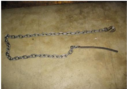
Choker chains are 4' to 6' in length, with a grab hook on one end and a pin on the other. The pin helps get the chain under the log. It works best if the pin has a slight curve so that it pushes up out of the dirt/duff on the other side of the log. The pin should be 8" to 12" long. The size of the chain must match the grab hook on the end of the winch cable and the notches on the back of the blade.
